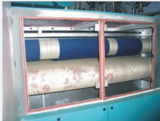
Chamber seal with silicon seal
